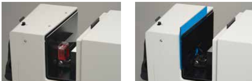
Sideless transmittance chamber for unlimited sample length (Maximum thickness: Approx. 50 mm).
