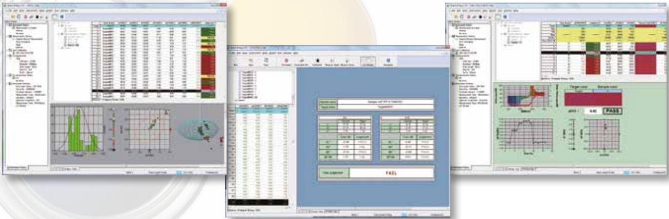
Layouts for screen displays and printed reports vary by application, from simple pass/fail assessment or statistical process control for production lines to detailed analysis for R & D work.
