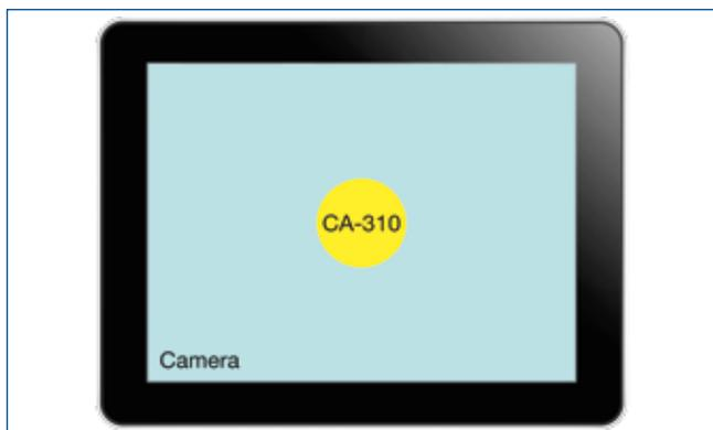
Figure 2: The yellow circle represents the CA-310 measurement spot, the blue area indicates the camera's field of view.
