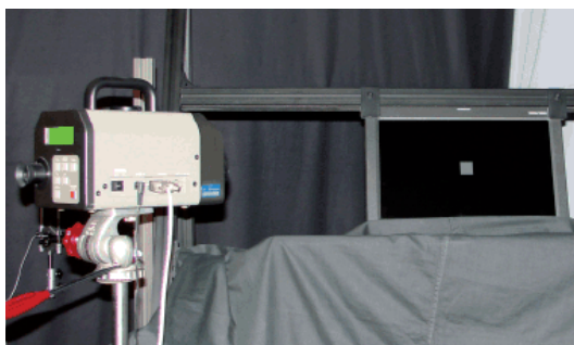
Measuring apparatus for determining the viewing angle dependence of the Konica Minolta CS-1000 spectroradiometer
