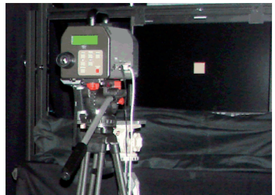
Chromaticity coordinate determination on 15 EBU colour charts with the Konica Minolta CS-1000 spectroradiometer
