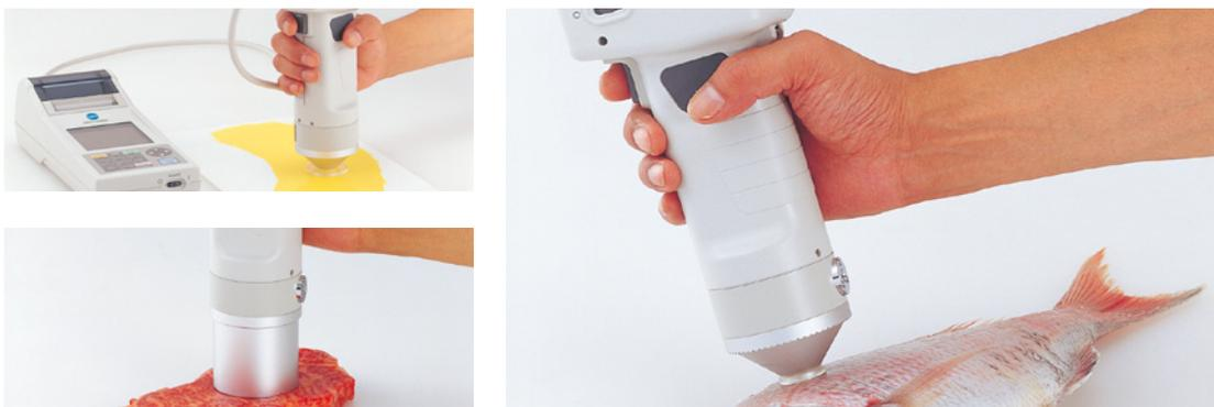
Konica Minolta portable Chroma-Meters have become a “defacto standard”, especially in the food and ingredients industry. The CR-400 and CR-410 represent a step forward in usability, portability, durability and reliability as well as flexibility in terms of sample forms including solids, paste, powder and granules. The instruments also offer either a small or large measurement area, to suit either homogenous or irregular samples.
